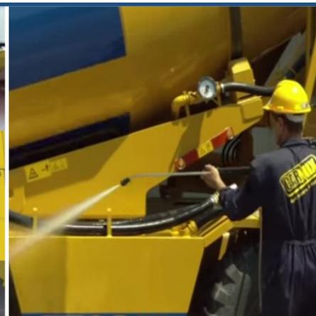
**Electrical high pressure washing system for better cleaning of the machine.**
