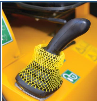
Joystick Operation for all main functions of loader for operators ease.
