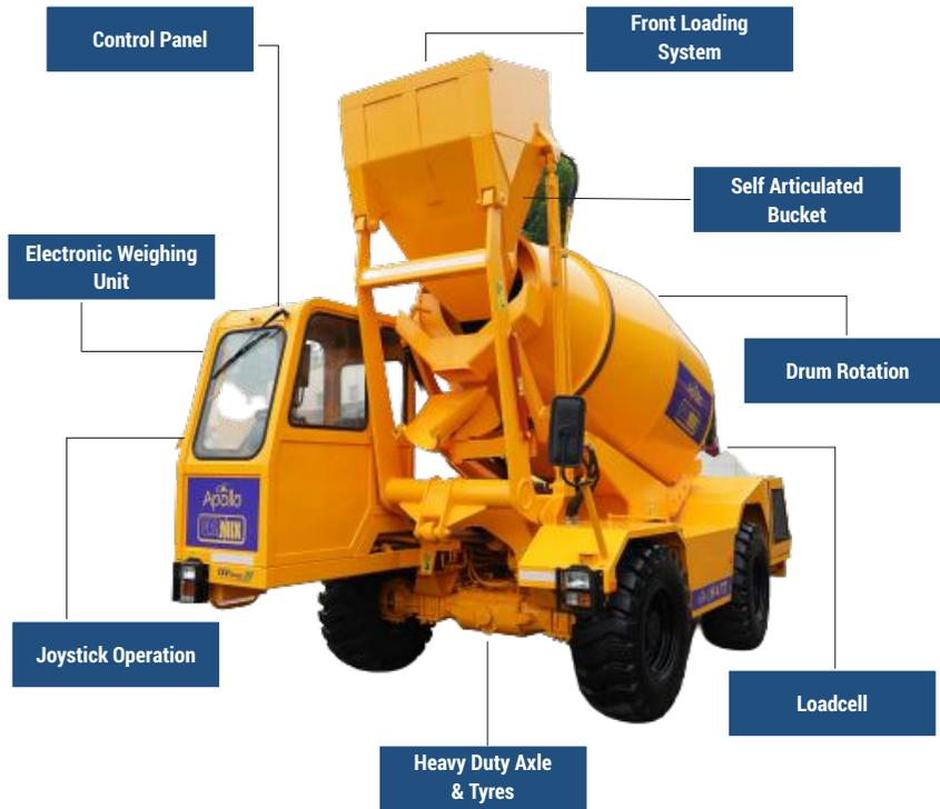
**INNOVATIVE A DIGITAL TECHNOLOGY ADVANCED LOADCELL WEIGHING SYSTEM – FOR A PERFECT CERTIFIED MIX DESIGN**
