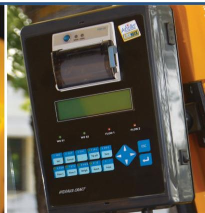
Electronic weighing system cum printer to get quality concrete as per mix design.
