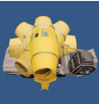
270° Drum Rotation to discharge concrete on all 4 sides of the machine.
