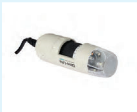
DINOLITE - AM 2111 Series (Digital Microscope) for wire inspection through Laptop and hand phone
