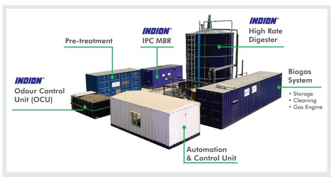
The above plant is designed to treat approximately 900 kg/d of organic waste generated by a community kitchen and 2 – 6 m³ of sewage sludge/d. It produces 20 KW/h of electrical energy and 1.35 tonne/d of organically rich fertilizer at full capacity. Similar modular systems are available for treating varying capacities of waste generated by hotels, residences & institutions.
