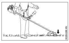
Mowing tools such as mowing heads, grass cutting blades and brush knives
