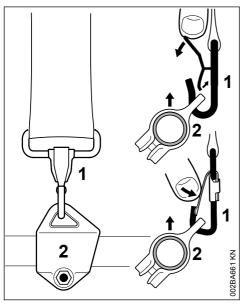
► Press down the bar on the carabiner (1) and pull the carrying ring (2) out of the carabiner.
