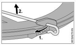
Disconnect wire rod from the transport guard.
