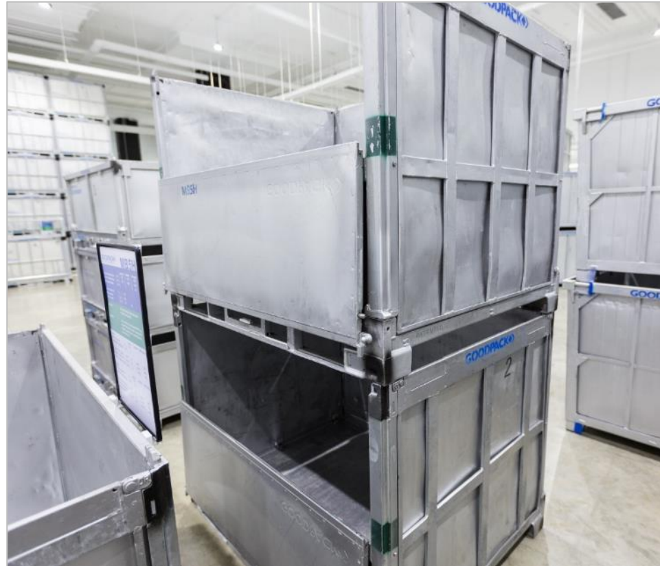
Two MB5H's stacked and exhibiting the foldable half-sidewalls.
